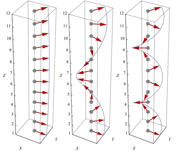
FIG. 1. Orientation, for a pure NESS in the Zeno regime, of the lattice spins of a driven  $XXZ$  chain arranged along the  $Z$  axis with boundary twisting in the  $XY$  plane for winding number  $m = 0, 1, 2$  (left to right). The  $Z$  labels indicate the lattice points along the chain. Parameters:  $N = 12$ ,  $\Phi = \pi/3$ .
