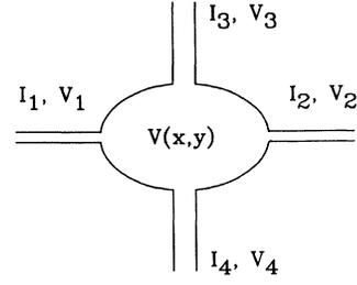
FIG. 1. Schematic picture of a four-lead two-dimensional conductor with the relevant potentials and currents.
